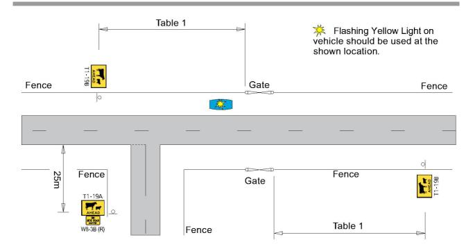
FIGURE 2 - Stock Crossing Site near an intersection
